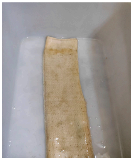
Figure 7. Immersion of the fourth sample in the sodium alginate solution.
